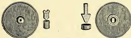
View of the Cap-chambers and Sections of Caps and Anvils of the "Eley" and "Life" Cases.
